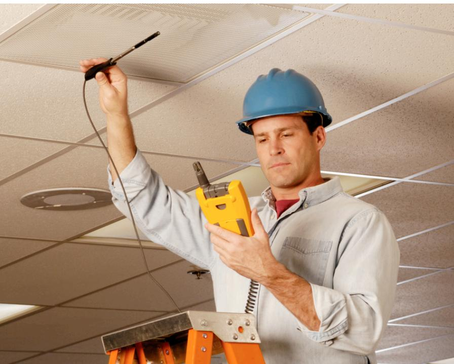
Measuring air flow at a supply register.
