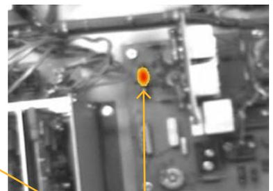
**Figure 6.** Color-alarm example with hot threshold set at 300 °F
