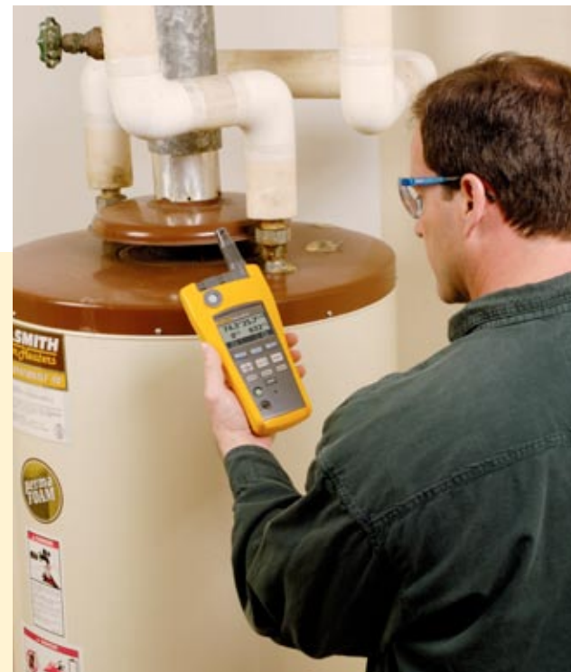
Measuring CO around a gas water heater.
