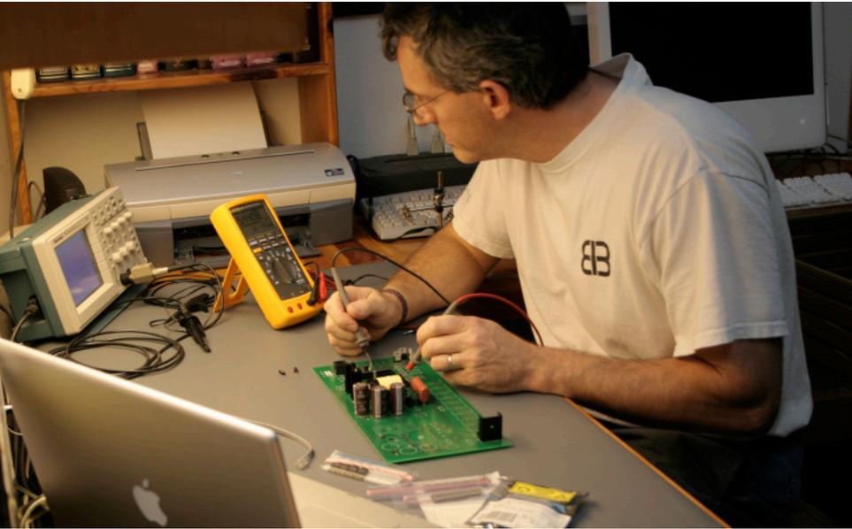
Bruce Leonard testing the Variable Spark Injection board for Engine Logic Systems LLC.
