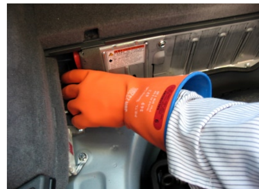
After putting on insulating gloves, the technician disconnects and removes the battery service plug. 2007 Toyota Prius hybrid shown.
