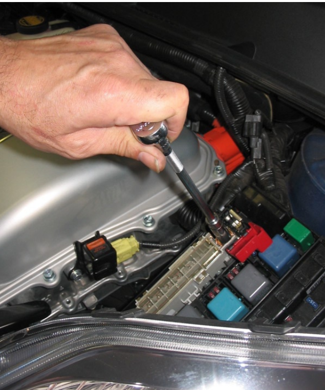
After turning the vehicle off, the technician disconnects the vehicle's auxiliary 12 V battery to ensure that the HV battery pack is mechanically isolated. The battery of this Toyota Prius can be disconnected from inside the main fuse/relay box.
