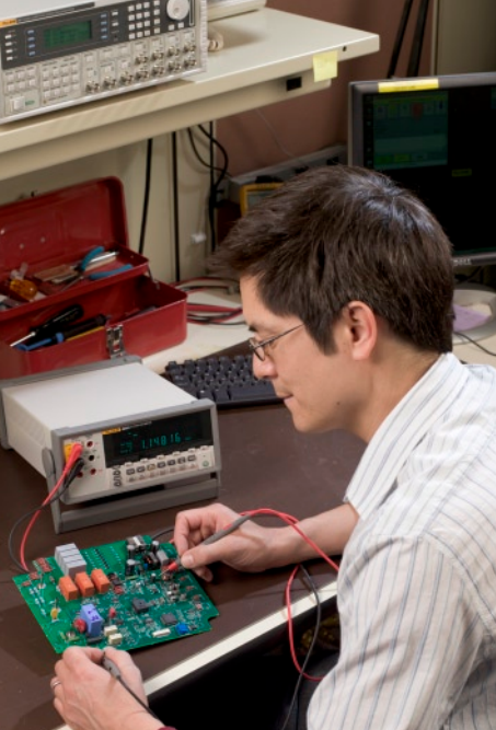
This otherwise complex setup, requiring a four-wire connection, is simple with the aid of the 8808A's patented split-terminal test leads. Each lead contains two conductors.
