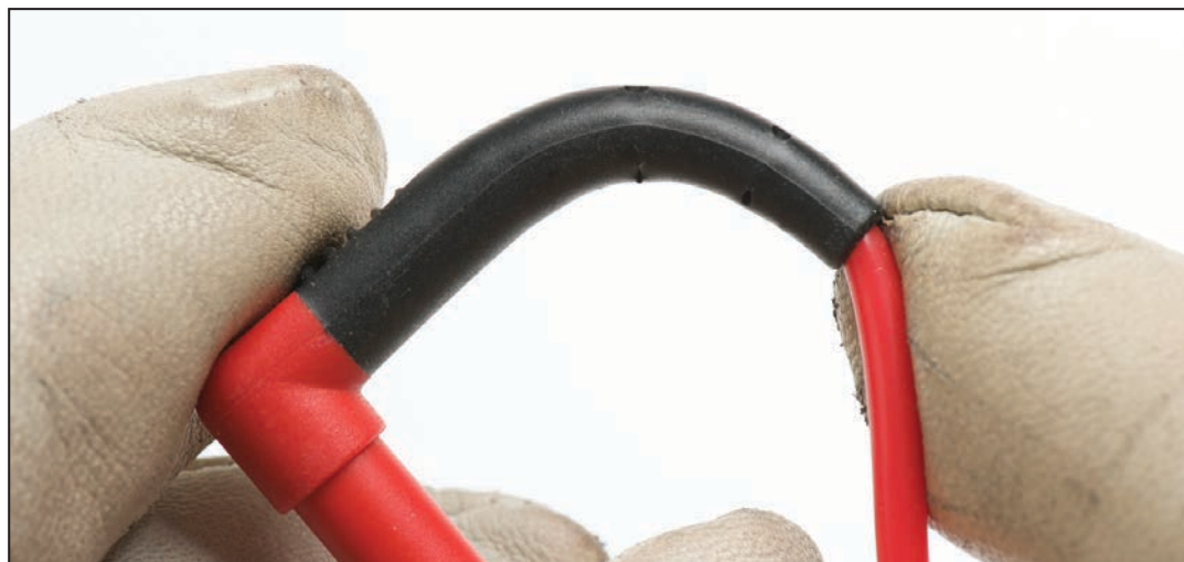
Test lead input plugs should bend without showing cracking in the insulation
