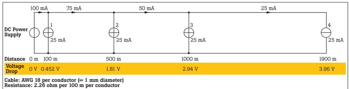
Figure 6: Calculation of voltage drops resulting from connected devices and their distances from the power supply.
