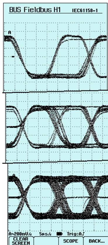
**Figure 8:** This series of Fluke 125 screens show how the trace builds up over successive acquisitions using the instrument’s eye-pattern display mode.
