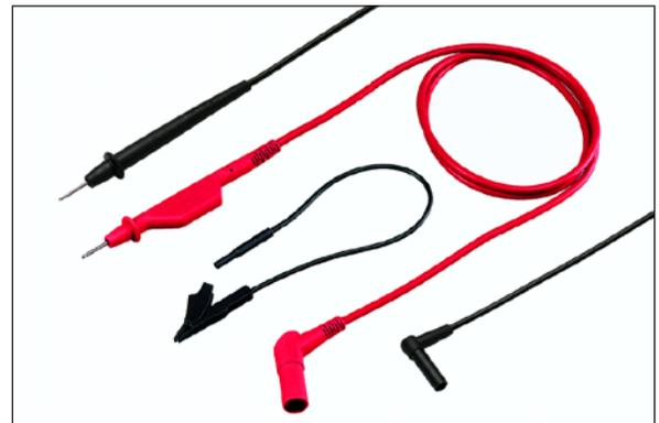
**Figure 2:** The STL120 (red) and TL75 (black) test leads are the primary tools for making test connections onto a FOUNDATION Fieldbus. When encountering heavy noise on the bus, try the shorter lead with the alligator clip (center item). All three items are standard with the Fluke 125 Scopemeter.
