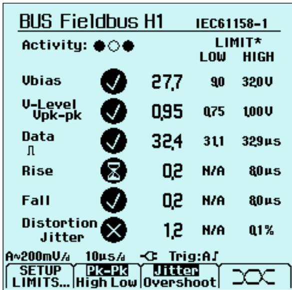
Figure 5: Fluke 125 screen showing results of a Bus Health Test.
