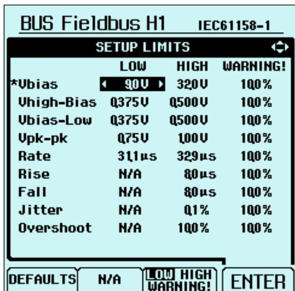
**Figure 7:** Set-up screen for changing test-limit values.
