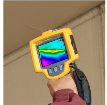
Thermal Imagers are becoming indispensable for identifying airflow and moisture problems and air leaks by their tell-tale changes in temperature. By using a thermal imager to scan a building, techs can quickly zero in on problem areas and then investigate further with other tools.
