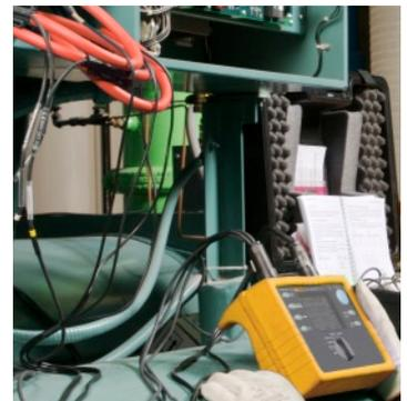
Many HVAC techs are finding that logging power usage of HVAC systems gives them the data they need to convince clients to upgrade to new, more efficient systems. This tech is using the Fluke 1735 Power Logger.
