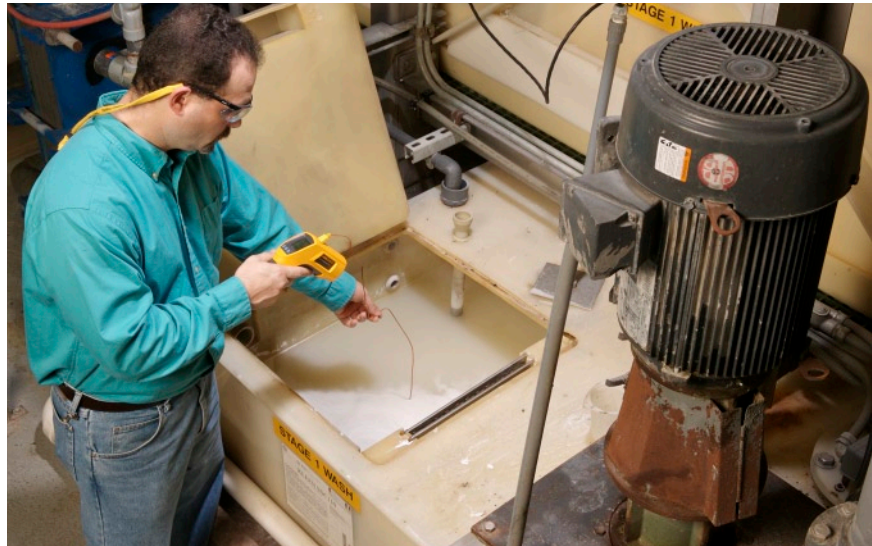
Mitch Curtin of Helios Coatings Inc., uses the 568 IR Thermometer and the included 80PK-1 Bead Probe to monitor the fluid temperature of a soap bath solution used in the cleaning of raw wheels before the first primer process.
