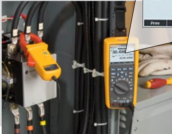
Phase current reading + motor speed using i1010 clamp
