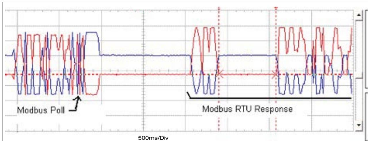
**Figure 1.** This data capture at 5 ms/div reveals both the poll and the response. Notice the delay of approximately 7 ms in the response.
