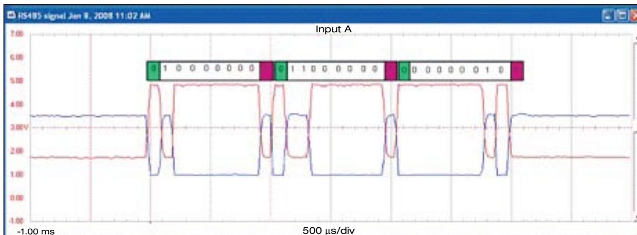
**Figure 2.** The data capture of the first three bytes of the Modbus RTU response at 500 μs/div. This representation includes a decoding of the response signal to clarify the slave node address, the function code and response data length in bytes (represented by the binary logic manually superimposed above the waveform).
