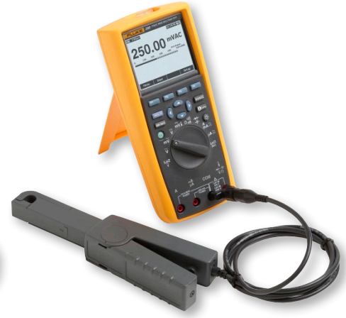
Figure 5: At 10 mV/A, a reading of 25 amps displays 250 millivolts.
