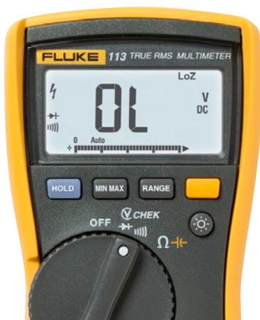
The Fluke 113 is now ready to make either a continuity test, diode check, or voltage measurement. All three tests are automatic. The meter will determine the correct measurement.
