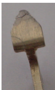
Figure 2a. Cracked contact face.
