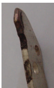
Figure 2b. Cracked face after fault.
