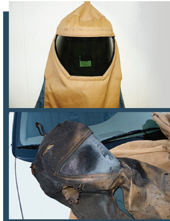
Figure 1. HRC4 Arc-Rated PPE, before and after an arc flash.
