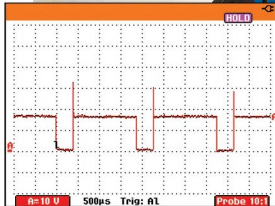
By adjusting ScopeMeter® test tool's trigger level, the technician can further isolate the causes of spikes.
