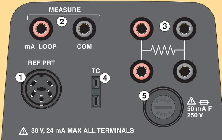
1. PRT Reference Thermometer 6-pin DIN Smart connector
