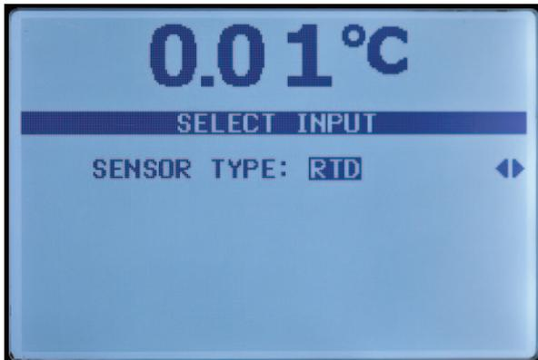
Use arrow keys to select mA (for transmitter), TC (for thermocouple) or RTD.
