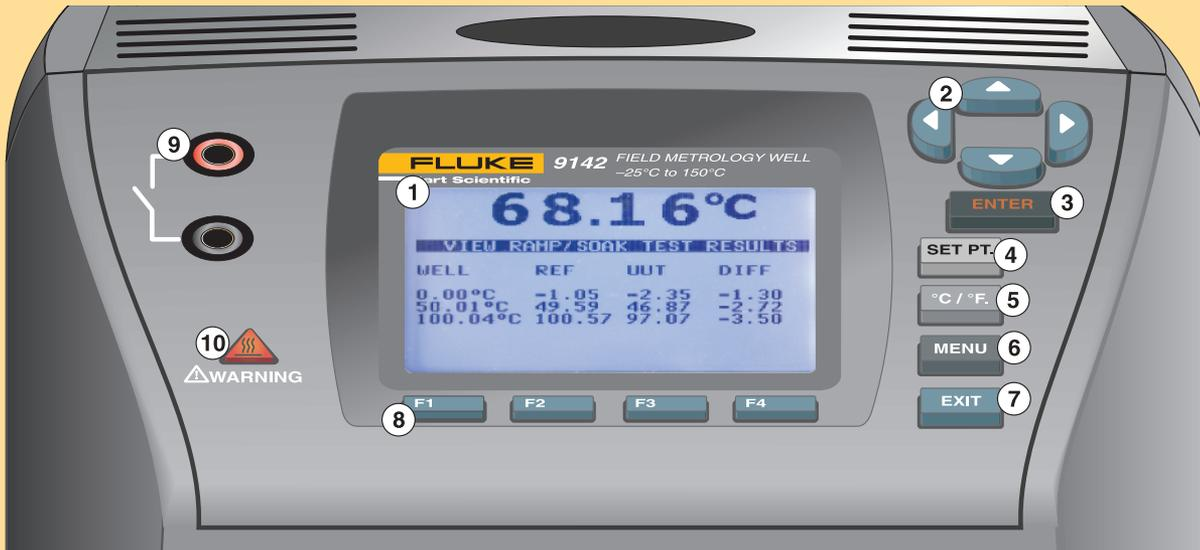
1. 240 x 160 pixel monochrome graphics LCD with backlight.
