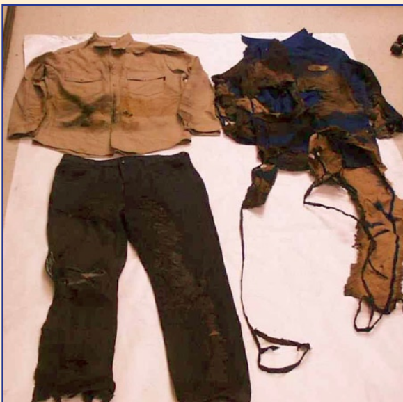
Figure 3. Arc-related break open of fabric "Two Similar Incidents; Two Different Outcomes."
