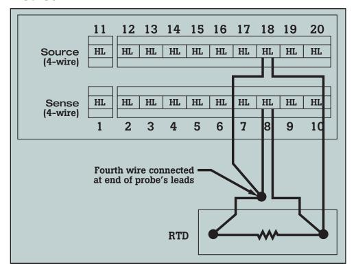
In cases where the connection to the 3-wire RTD is extended with wiring between the inputs and the probe leads, Method B should be used. This prevents the resistance or temperature changes of the added wiring from causing additional errors in the temperature measurement.
