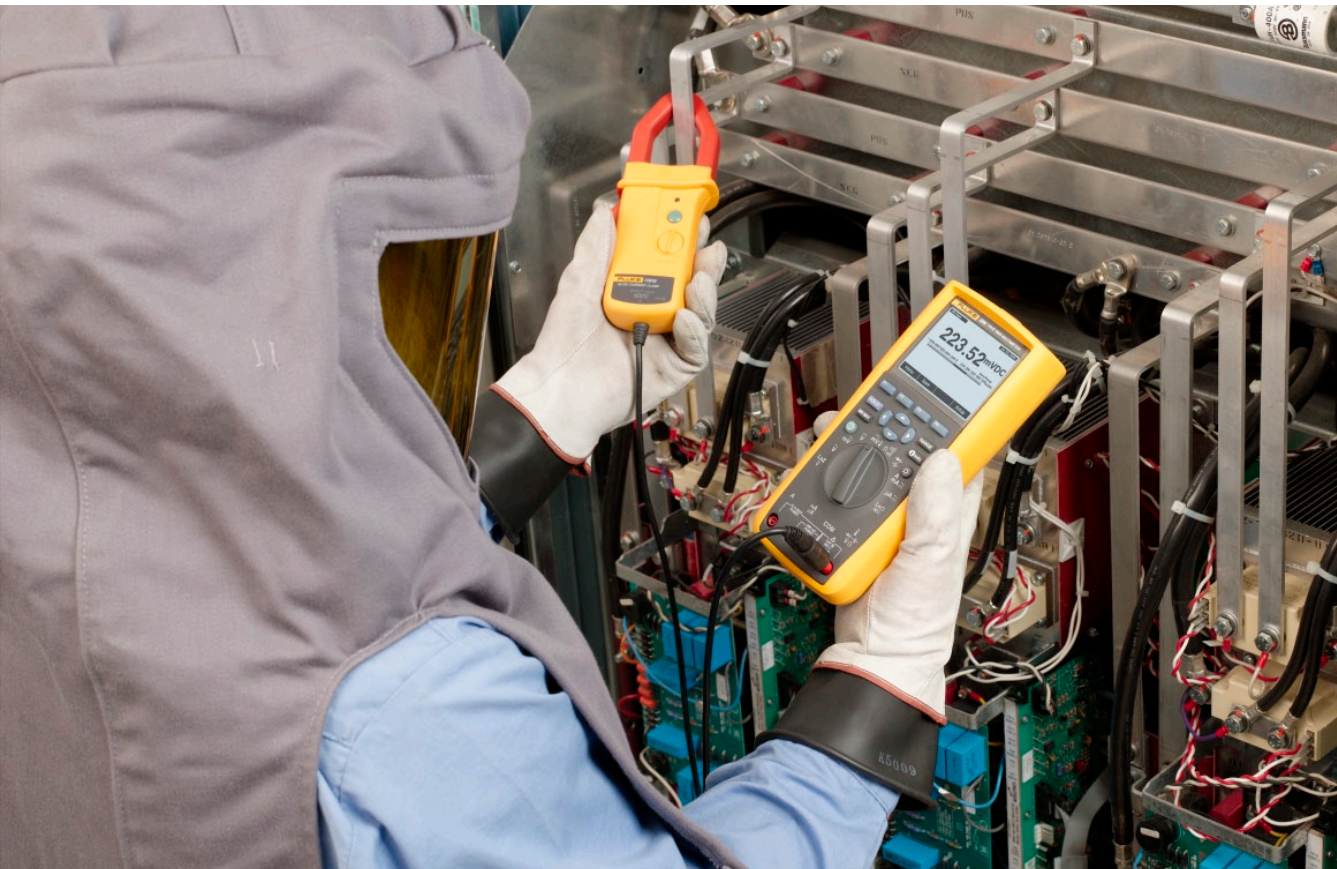
Hazard/Risk Category 2* now requires either a switching hood or a balaclava hood and arc-rated face shield combination.
