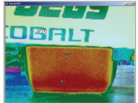
Figure 3. Merely towing the JEGS.com racer car from the pits to the inspection area and back heated this drag slick by 15 °F
