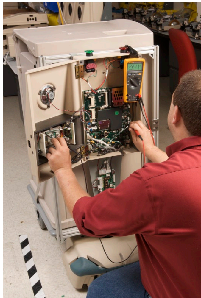
Troubleshooting controls on the tow-unit that the robot pulls.
