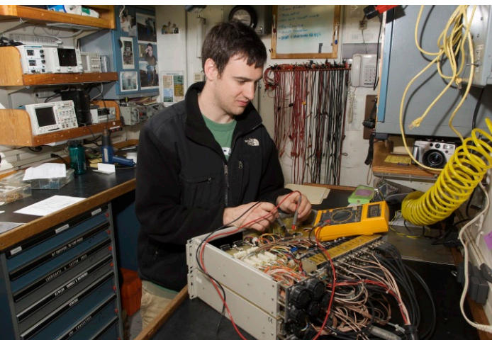
Sean Kelley at the bench in Alvin's work shop. He's troubleshooting an electrical problem on a 26 V dc video controller that is very valuable to each dive but is vulnerable to conditions on the sub.
