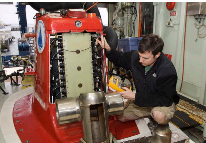
Kelley double checks the continuity of a video camera connector that was just installed on the sub's top side, before the access panel is closed back up.
