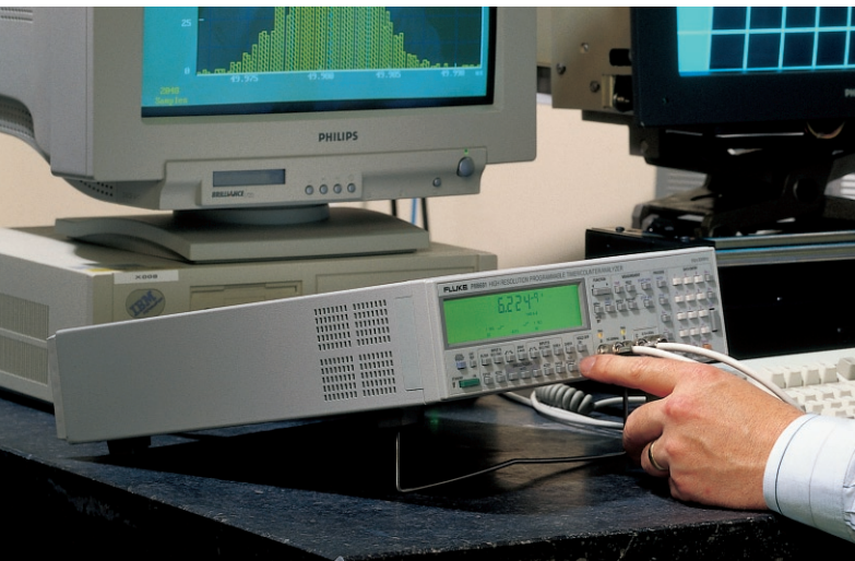
Using MET/CAL® software to automate the calibration process.
