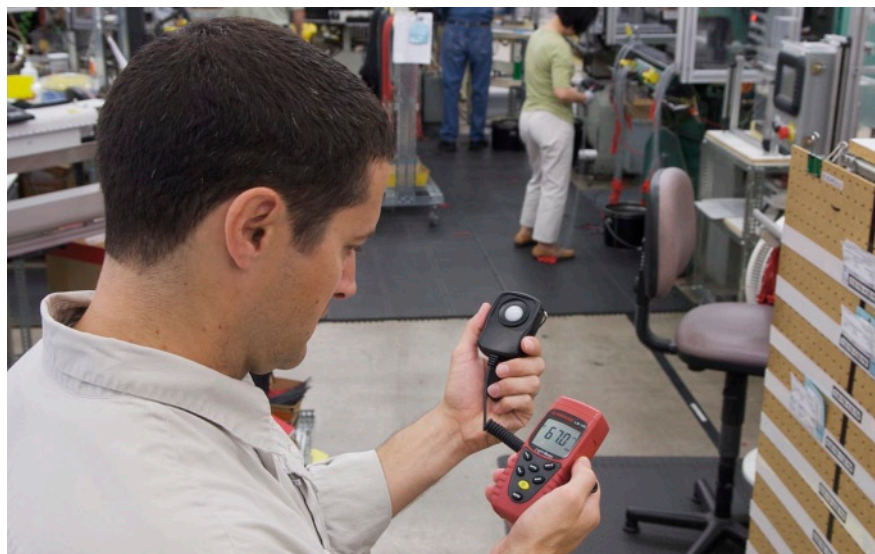
Use a light meter that allows you to select footcandles to measure illuminance.
