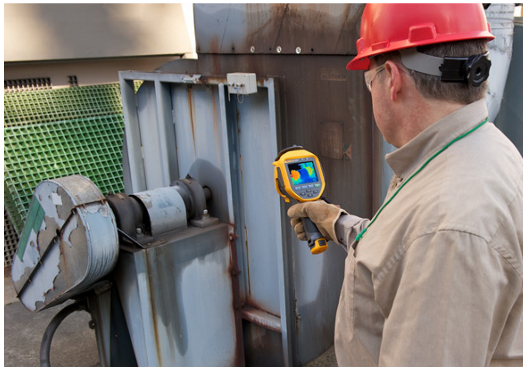
Shafts made of shiny stainless steel can be tricky to measure with thermal cameras. Compensate by measuring close to the coupling.
