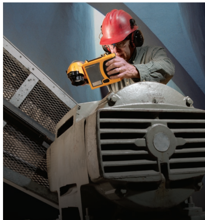
Scan the components of rotating equipment, especially the bearings and shaft. Watch out for shiny metal that can throw off a thermal reading.
