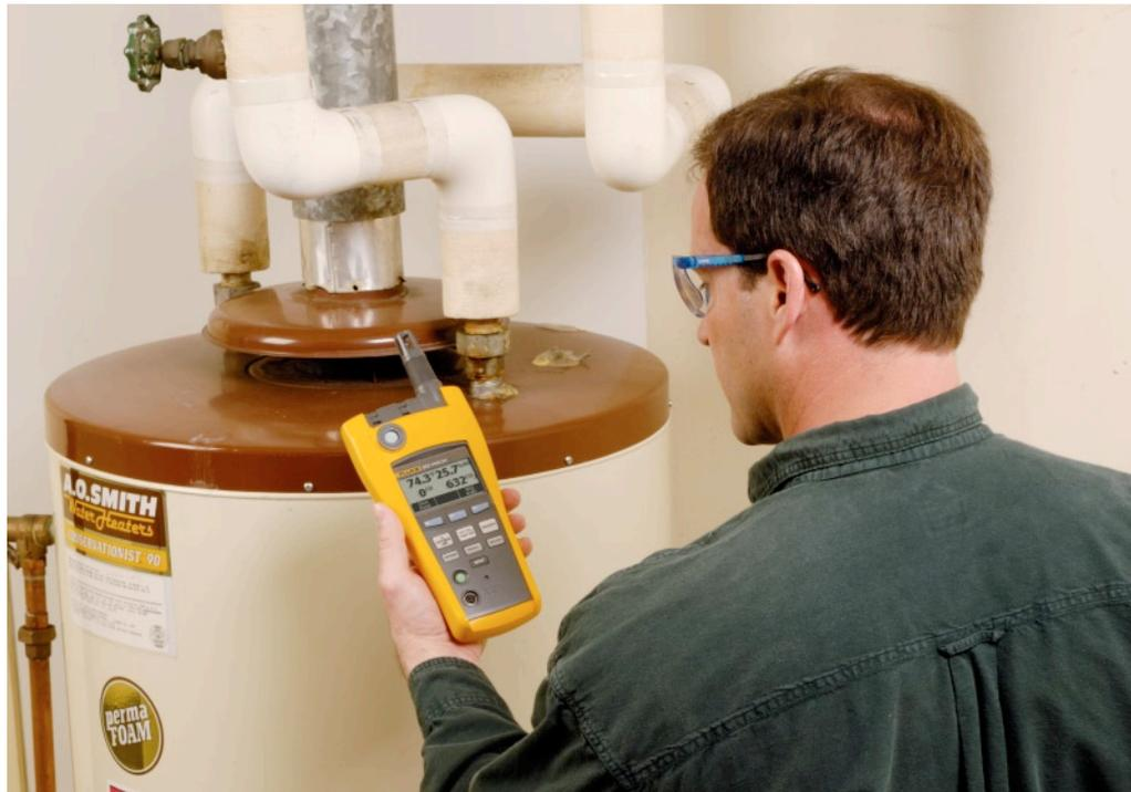
When taking readings near any combustion equipment, measure not only CO but CO<sub>2</sub> and temperature as well.
