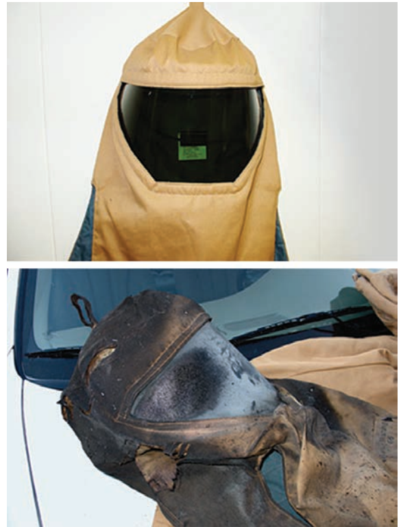
Figure 1. PPE Category 4 arc-rated clothing and PPE before and after an arc flash.
