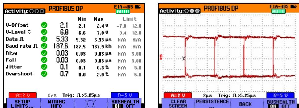
Figure 2. After making corrections to the Profibus network, new screen images of the Bus Health parameter screen (left) and the eye-pattern screen (right) were recorded. These clearly show improved network performance, with all parameters meeting requirements and well formed square wave pulses.
