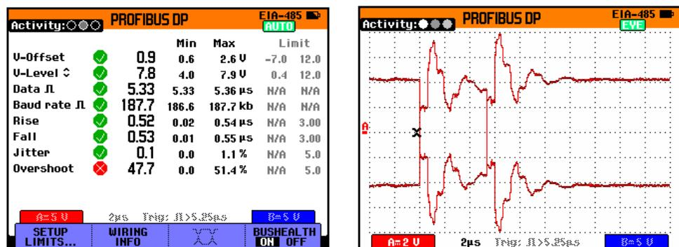
Figure 1. Left: The overshoot reading at this station is so high that an error in the network is likely and calls for further investigation. Right: The alternative way of looking at the bus signals using the eye-pattern mode shows that pulses are largely distorted, making it clear that there is an aberration on the signal at this location.
