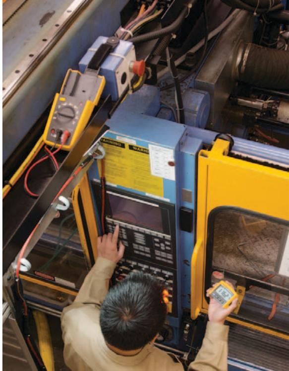
can make it possible to physically separate the tasks of positioning your meter and reading test results, so you can devote full attention to each task—and reduce the hazards.
