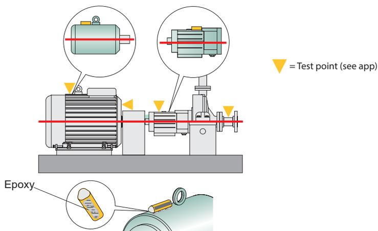
**Q 11:** Where do I mount the sensor on the bearing?
