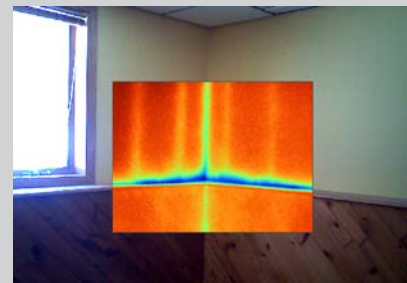
Picture-in-Picture, an IR-Fusion viewing mode, takes the guesswork out of re-locating problems by providing a frame of reference such as in this infrared image of an air leak at the point where an exterior wall meets the foundation.
