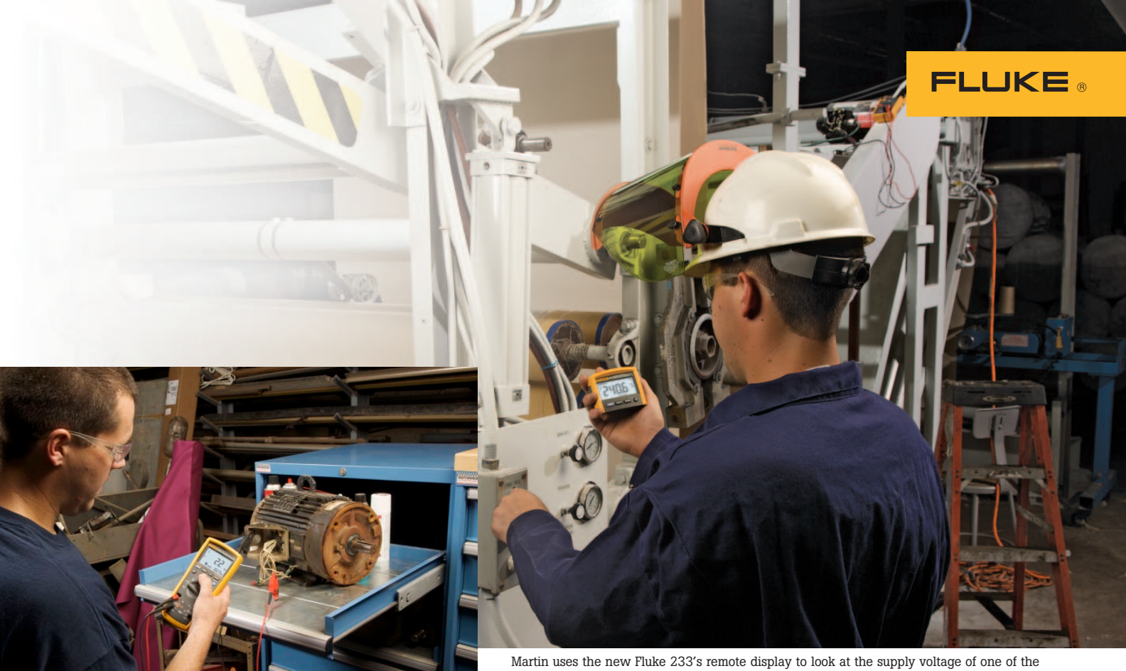
Martin uses the new Fluke 233's remote display to look at the supply voltage of one of the drive motors on the textile spooling machine. The remote display allows him to work at a safe distance from the moving machine parts and live voltage. To operate this machine and monitor live voltage would have been a two person job in the past.
