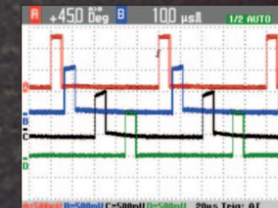
Measure time or amplitude relationships of 4 test points simultaneously
