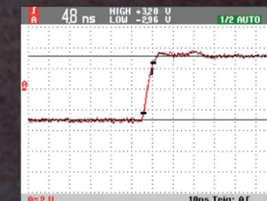
500 MHz with fast sample rate accurately capture and displays edges of pulse width modulated signals or harmonic content in fast clocks signals
