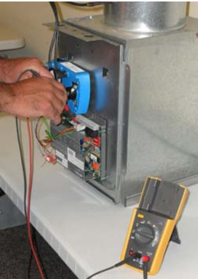
The main section of the 233 meter stays in place while the technician uses the detachable display to check results elsewhere.
