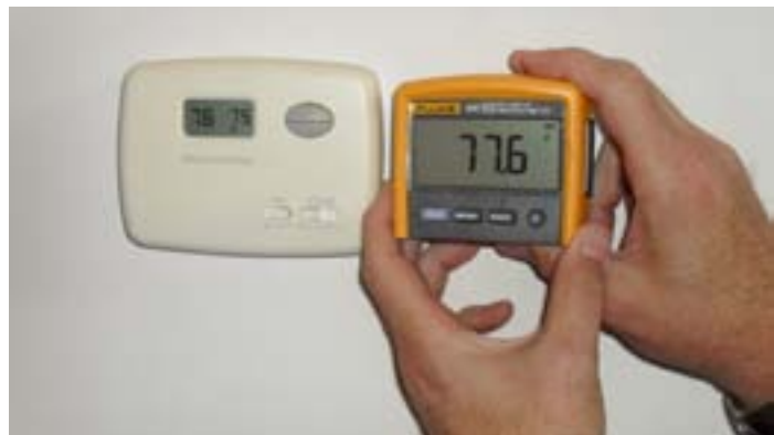
A technician can compare the results on the 233's detachable display to the reading on a remote thermostat.
