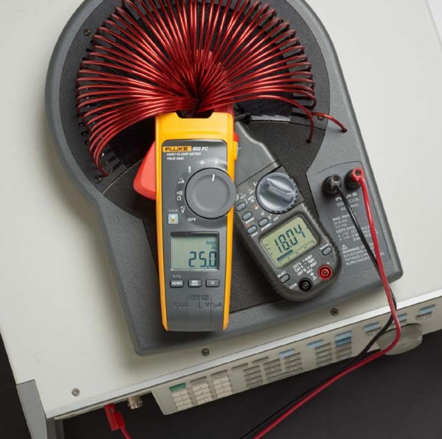
One current—two readings. Which do you trust? This demonstration shows a non-sinusoidal waveform passed through a coil. The true-rms clamp meter shows an accurate current reading. The averaging responding clamp shows a reading more than 25% low.
