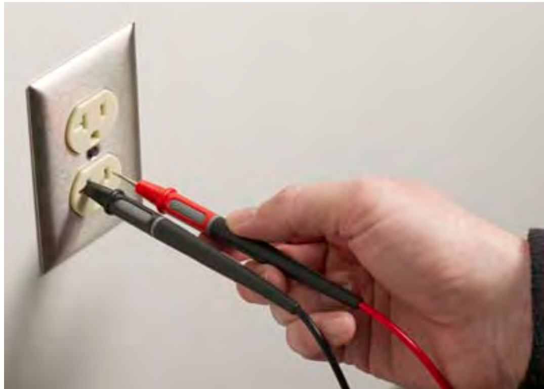
Fluke's new TL175 TwistGuard™ test leads let the user select the proper tip exposure for the job at hand. Test leads are a small item that can have large safety and productivity implications for test equipment users.
