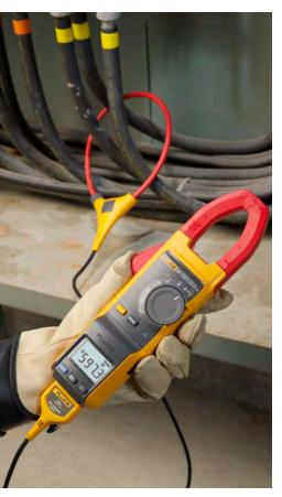
their associated dc circuits with a high-quality digital multimeter (DMM) with an amp clamp or a clamp meter with voltage-measurement capabilities.
