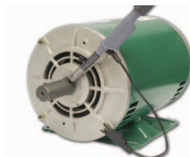
Measuring motor shaft voltage with an Aegis shaft voltage probe (Photo courtesy of Electro Static Technology).
