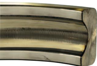
Fluting of a bearing race caused by bearing currents (Photo courtesy of Electro Static Technology).
