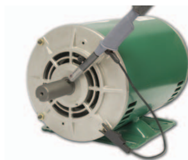
Measuring motor shaft voltage with an Aegis shaft voltage probe (Photo courtesy of Electro Static Technology).
