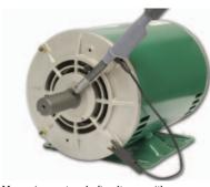
Measuring motor shaft voltage with an Aegis shaft voltage probe (Photo courtesy of Electro Static Technology).
