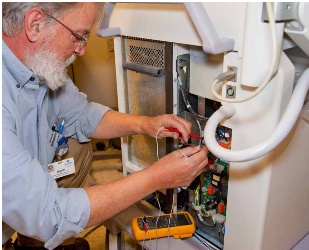
Brian Morey, B.S., CBET, Summa Western Reserve Hospital Biomedical Equipment Technician/Imaging Specialist, checks the power control PCB for a C-arm interlock "good" signal. That enables the ARCNET nodes that control the C-arm.
