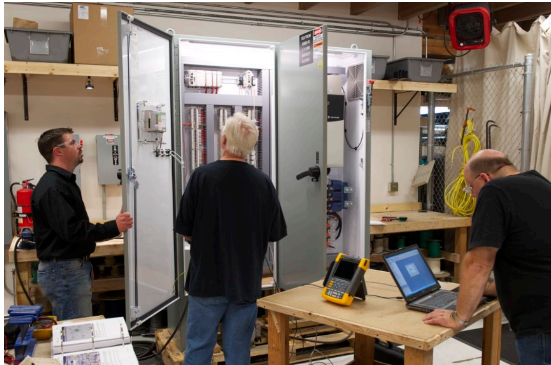
Zack Bryson and Jerry Katona examine the operation of the low-voltage side of the dust collector control panel while Kim Kruckenberg sends test commands from his laptop.
