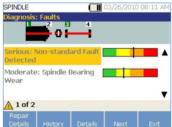
Under certain conditions, the Fluke 810 Vibration Tester may identify a "nonstandard fault."
