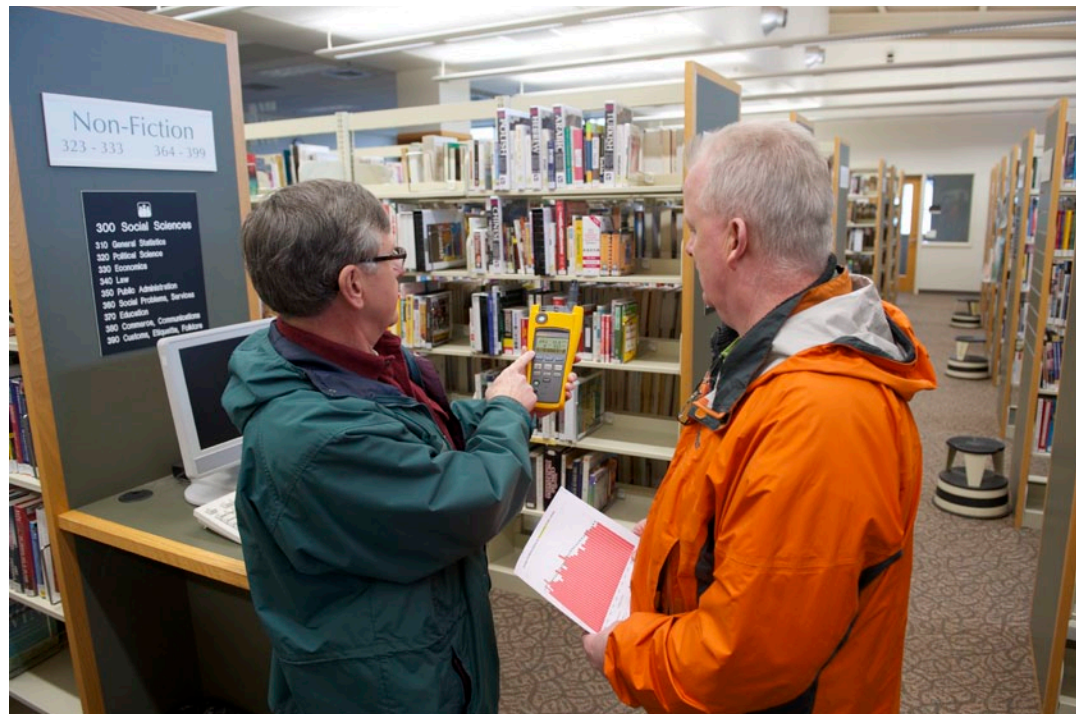
Boge and Pittis use the Fluke 975 AirMeter™ tester to spot-check air quality in the Anacortes Public Library.
