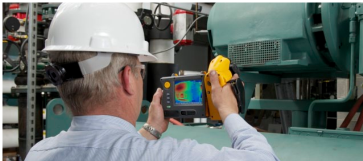
Bernie Kargol uses a Fluke FlexCam® thermal imager to look at the thermal signature of a motor on a chiller.
