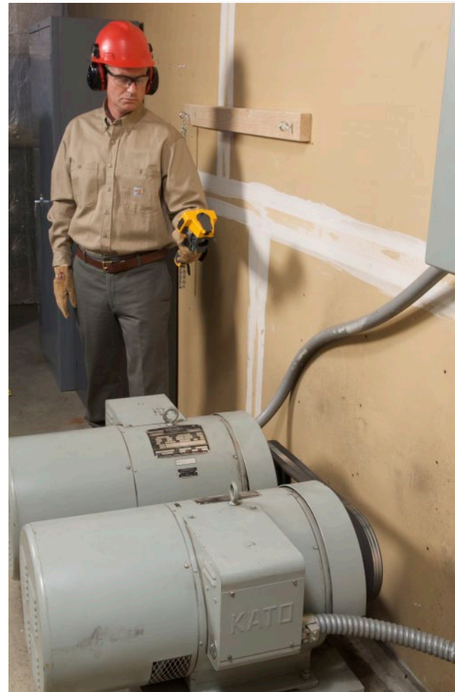
Infrared emissions from electric motors may reveal issues with bearings, drive components and overall performance.
