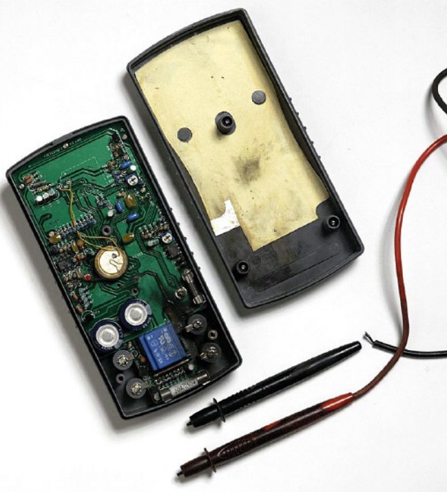
Failed digital multimeter and probes that were not certified by an independent rating agency.
